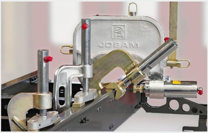
Our product line of C-clamps for pressing and riveting is unique and the different versions are well-suited for repair and bodywork on heavy vehicles. The clamps can be used as a complement regardless of the available equipment in the workshop. The offer includes small 10 ton C-clamps for minor local deformations up to 40 ton C-clamp that can be used for both pressing and riveting.
